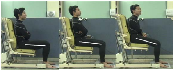
(a) 7 degree (b) 14 degree (c) 21 degree Figure 4. Initial height of seat plate based on initial femoral angle.
